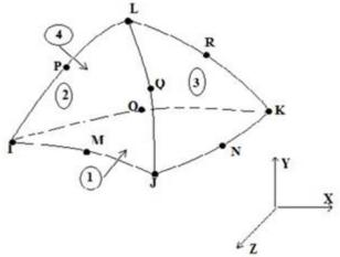
Fig.1 10 noded Solid187 element
