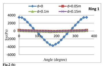
Fig.2 (b) Fig.2 Distribution of  $S_z$ ,  $S_{yz}$  and  $S_{xz}$  respectively, along the ring of radius=0.2m for various sizes of delamination
